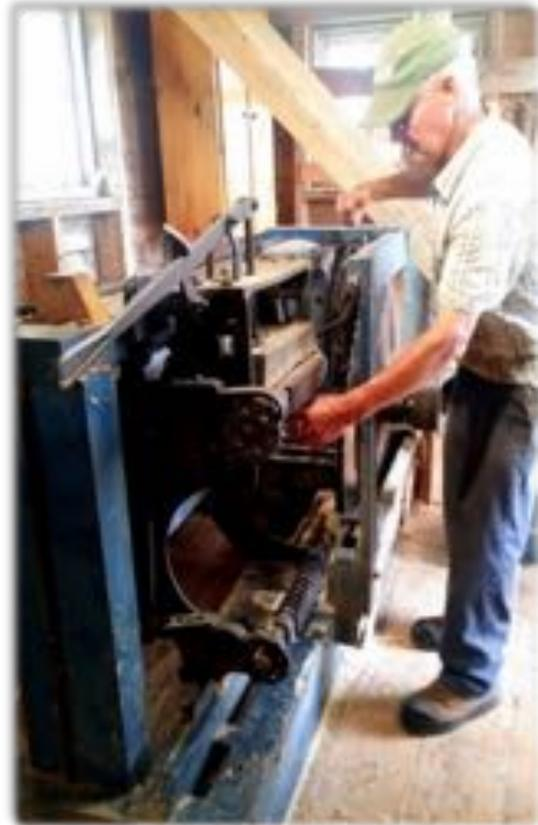
Once powered by water mills and steam, the mills and planer are now run by PTO and belt. A laser guide has been installed and a blower has been built to remove sawdust on the saw, but most of the original mill is intact.
