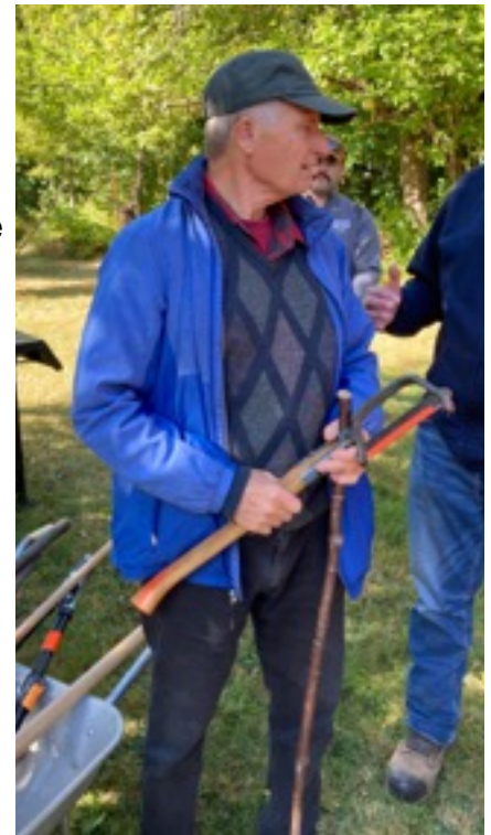
Bruce McCallum holding his Swedish brush axe. Note the D-frame extensions protecting the blade
